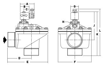
Fig. 3: External threaded type - aluminium
