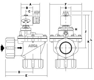
Fig. 2 Compression type fitting - aluminium
