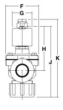
Fig. 1: Threaded pipe connection - aluminium
