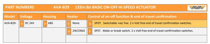
NOTE: US STANDARD STOCK IS WITH WIRING 'B', ALL OTHERS ARE FACTORY OPTIONS. DETAILS ON REQUEST.
