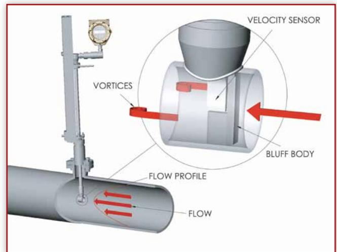
Insertion style vortex meters measure flow by detecting the local velocity at a strategically located position within the pipe. Using local velocity, calculated by measuring the rate at which vortices are alternately shed from a bluff body within the sensor, the AX2300 uses parameters such as fluid type, pipe size, and Reynolds number to calculate accurate measurements.
