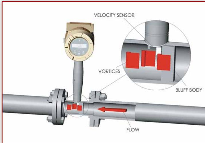
The AX Series of Vortex inline flowmeters measure flows of liquid, gas, and steam by measuring the rate at which vortices are alternately shed from a bluff body; this rate has been shown to be directly proportional to the flow velocity.
