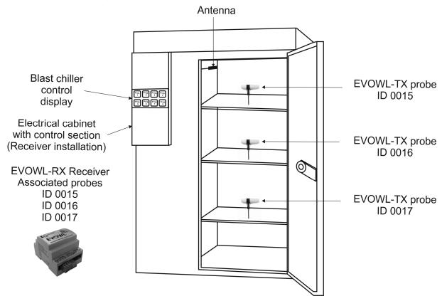
In the example above, 3 EVOWL-Tx probes with ID 00015 / 0016 and 0017 are installed, associated to the receiver mounted in the electrical panel. With the aid of the data received from the EVOWL-Rx receiver, the control section is able to monitor the product core temperature readings of the three EVOWL-Tx probes on the various trays on the trolley and inform the operator about the status of the blast chilling process by means of the display.
