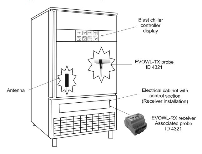
The example shown above is the typical with a EVOWL-Tx remote probe installed inside a blast chiller, with the receiver installed on a DIN rail in the control panel.
