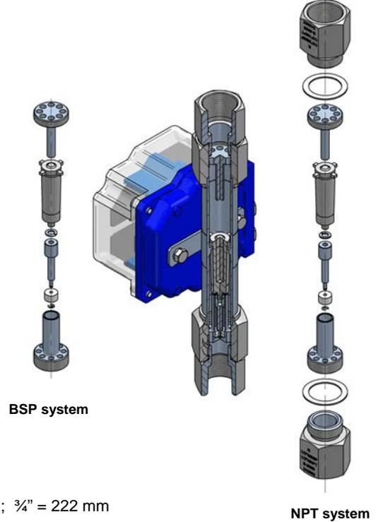
Total length M21 with damping system NPT: ¼" = 186 mm ; ½" = 212 mm ; ¾" = 222 mm
