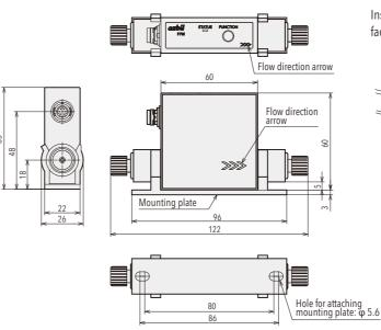
\*1. Mounting screws are not included (specification: screw head height of 5 mm max.).
